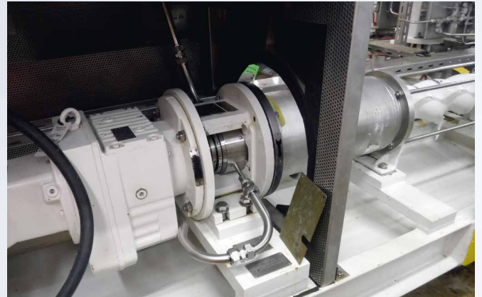
Seepex displacement pump sealed with Cartex-DN dual seals.
